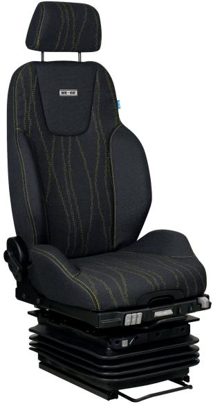
The BE-GE 3700.39 series is an air suspended seat with a separate suspension system. The seat's upper part 3700 has an extra low built profile as along with the suspension package 3909 are very suitable for construction machines and similar vehicles where armrests and vehicle controls are fixed between the seat's upper- and suspension unit.
